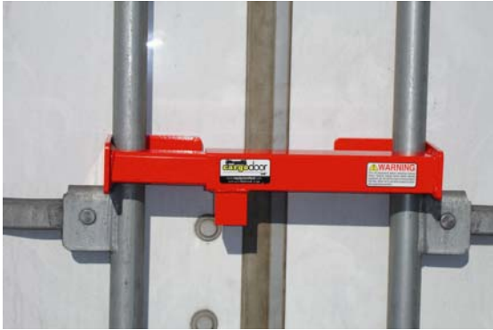
Cargo Door Lock (Weight 6 lbs) Built with 1" and 1.25" tubing having 11 gauge walls End Plates are 3/16" X 2"
